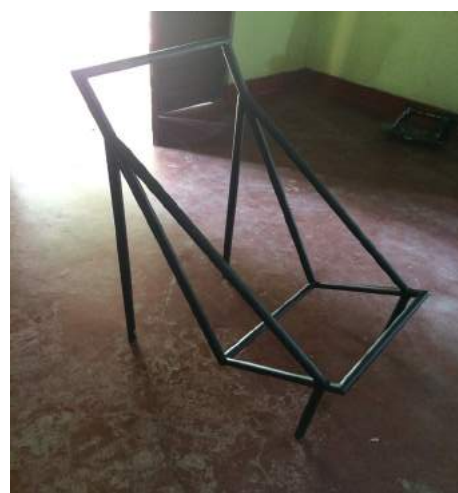
Above: a metal frame for use in making a titled bathing seat. Note the 90 degree seat is tilted back approximately 45 degrees to provide additional support.
